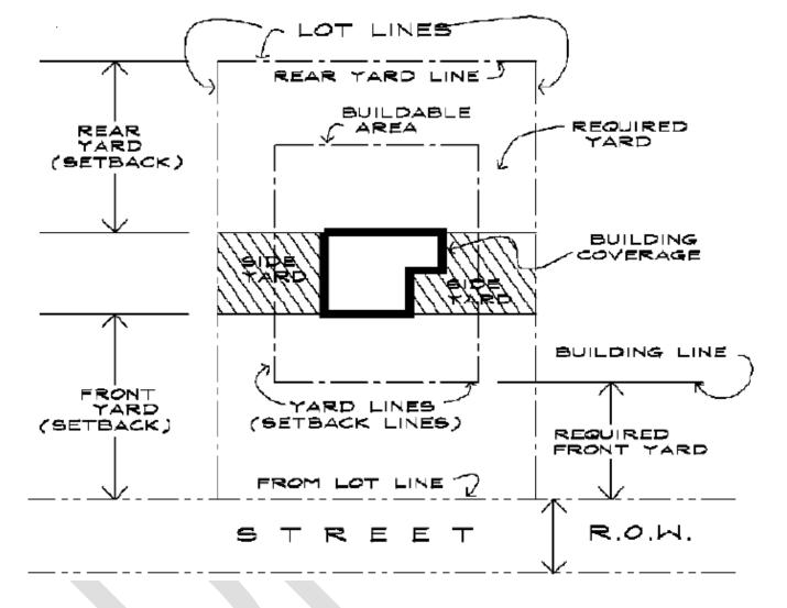
Figure 240-1 Setbacks, Building Coverage, Building Lines
